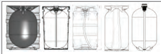
Figure 1.4. Examples of single-use keg configurations.
