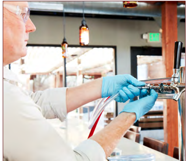
Figure 7.14. Ensure that all hoses are connected securely before cleaning.
