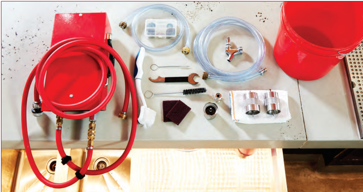
Figure 7.9. Recirculation pump equipment.
