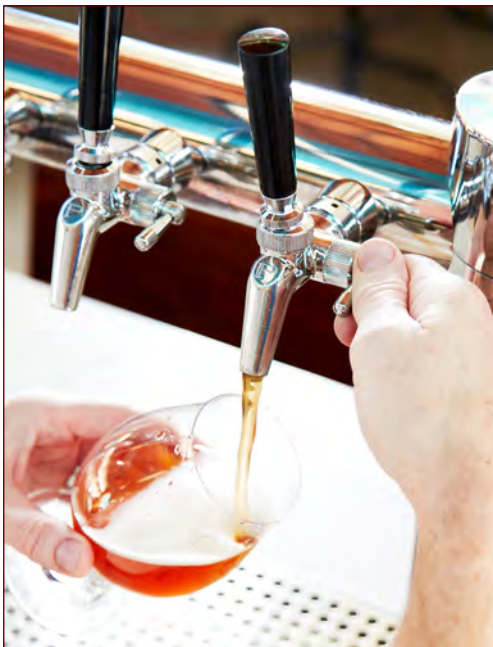
Figure 4.15. A flow-control faucet allows the bartender to maintain a manageable flow rate for highly carbonated beers.
