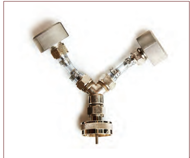
Figure 7.22. Cleaning flusher coupler connectors allow two different coupler systems to be connected. Shown here is a flusher that allows a “D” or “S” system to connect to a “U” system coupler.
