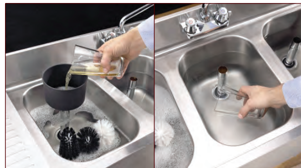
Figure 6.2. Left: In the three-tub sink system, residual beer must be poured to a drain, not the cleaning water. Right: Glasses are rinsed in the second tub between detergent and sanitizer tubs.
