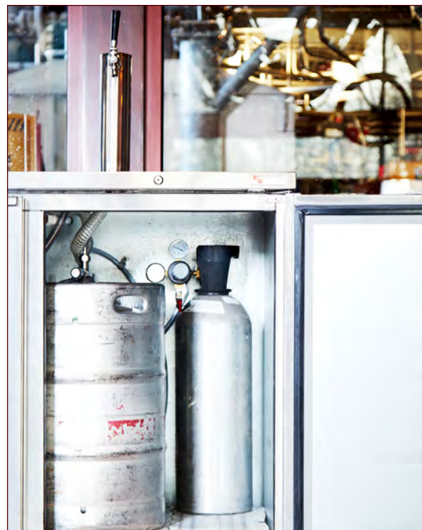
Figure 3.9. Direct-draw kegerator with single tower.
