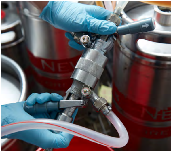
Figure 7.12. Couplers can be linked to aid in recirculation cleaning.
