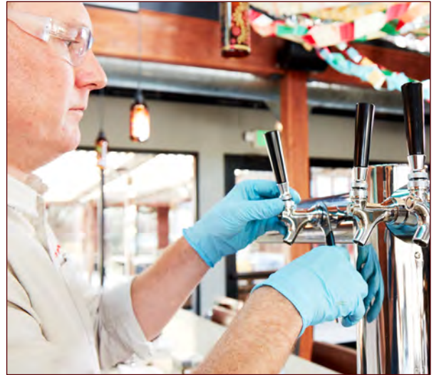
Figure 7.13. Faucets should be removed and cleaned separately.
