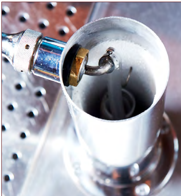
Figure 1.16. Bent tube shank installed in a single-tower kegerator.
